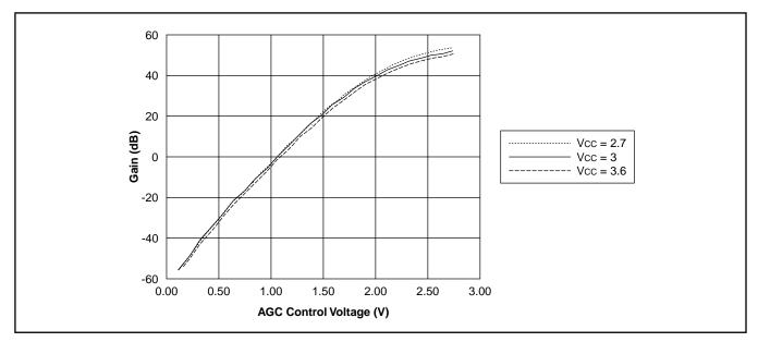
Figure 5 - CDMA Gain v AGC Voltage
