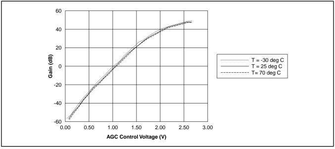
Figure 3 - CDMA Gain v AGC Voltage
