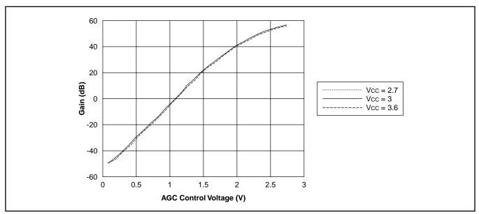
Figure 6 - FM Gain v AGC Voltage
