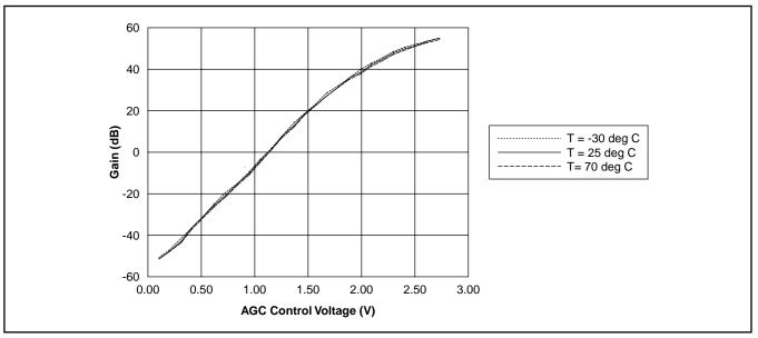
Figure 4 - FM Gain v AGC Voltage
