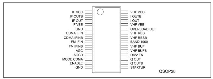
Figure 2 - Pin Connections
