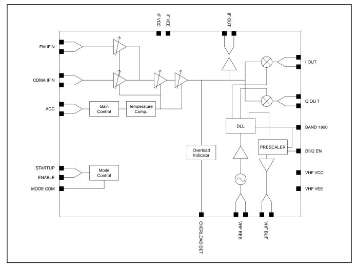
Figure 1 - Block Diagram
